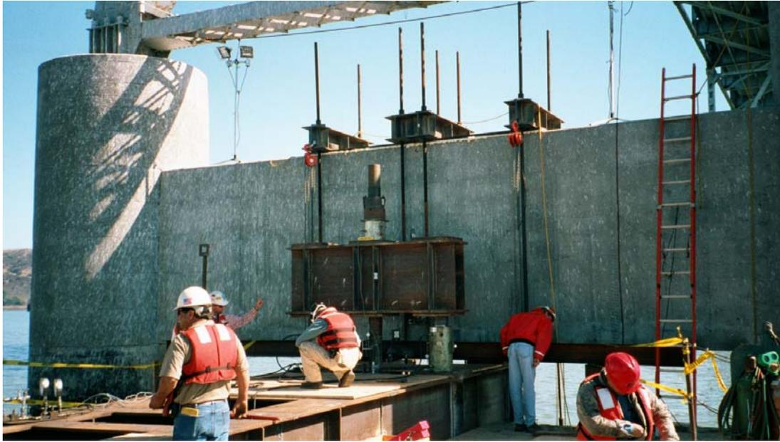
**Figure 6.** Performance Pile Load Test Setup
